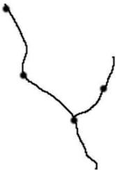
Drill a series of injection ports in the center of the crack. These ports should be drilled in a downward direction. Seal the crack with removable, non-staining clay, sealant, or caulk.
