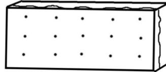
Drill a series of injection ports in a square configuration (90° angles) on the face of the substrate to create a "drill frame". Ports should be drilled in a downward direction. Wash the surface and interior of the crack using clean water to remove dust and loose debris. Any dust or debris remaining between the layers will impede the flow of the grout. If this is the case, more holes will be required to attempt to fill all hollow areas.
