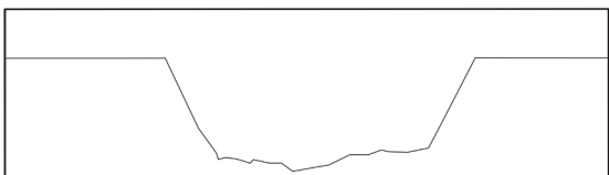
Incorrect (Feathered Edge) Surface Preparation
