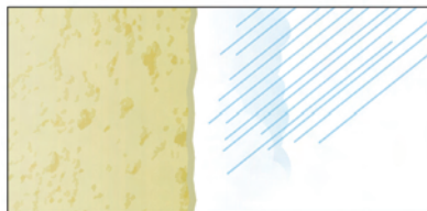
Phase 4: Powerwash to remove residue from pores
